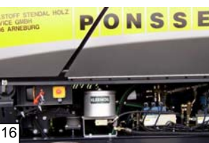
□ 1 – 3 KLEENOIL filter rigs in use in the factory for cleaning the system from fabrication residues; □ 4 – 6 KLEENOIL 24-Volt filter rigs in practical use; □ 7 – 8 KLEENOIL 24-Volt filter rigs in permanent use; □ 9 – 10 KLEENOIL filter rigs in industrial use; □ 11 – 14 KLEENOIL By-pass filter for motor oil filtration in utility vehicles, construction machines and stationary motors □ 15 – 18 KLEENOIL By-pass filter for filtration of hydraulic oil.
